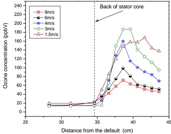
Figure 3: Ozone profile inside and out of the stator core at 8kV and varying air flow.
