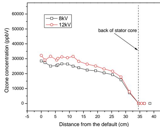
Figure 2: Ozone profile inside and out of the stator core without ventilation.
