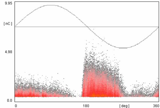
Figure 9 : PRPD pattern recorded on generator 5 of Shipshaw.
