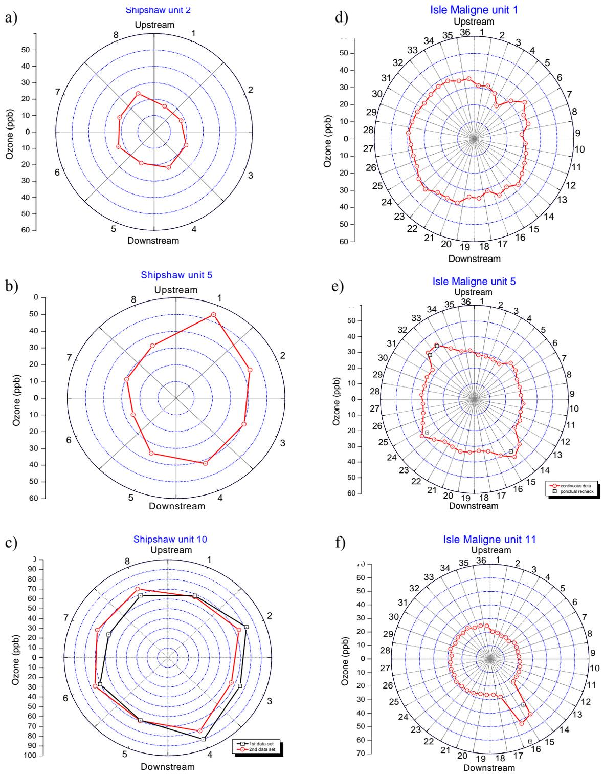
Figure 7: Examples of ozone distribution around generators.
