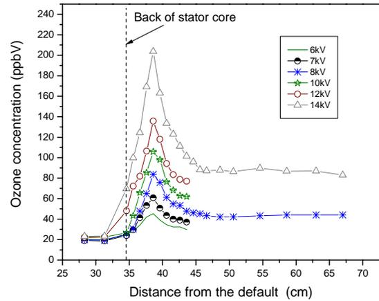
Figure 4: Ozone profile inside and out of the stator core with an 8m/s air flow and varying tension applied to the front bar.
