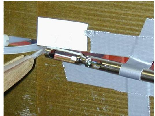
c) Back view: flow sensor and sampling tube
