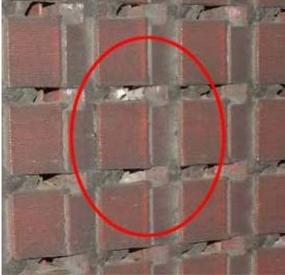
Figure 8: White powder from slot discharge, Shipshaw unit 10, position 5 o'clock.
